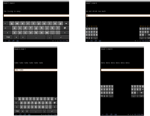
Figure 6. Left: unimanual gesture keyboards. Right: bimanual gesture keyboards.
