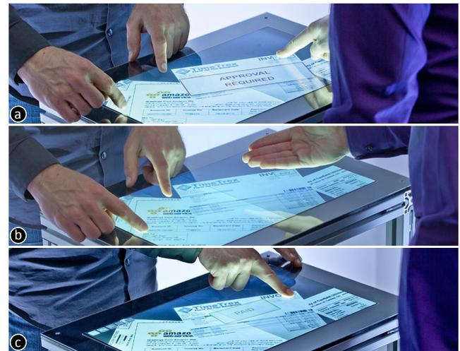
**Figure 4:** Example scenario. A bank manager (left) and clerk (right) approve invoices. (a) When the clerk encounters a bill above his approval limit, Fiberio refuses the payment. (c) The manager completes the transaction, pushing the same button.
