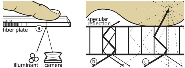
**Figure 10:** (a) The illuminant shines light onto the fiber optic plate. (b) A portion of the incoming light is reflected at the top of the fiber, traveling back down the fiber, where the camera observes it. (c) A fingerprint ridge touching the fiber, in contrast, frustrates the reflection at the top end of the fiber, so that only little light travels back down the fiber, causing this spot to appear dark to the camera.
