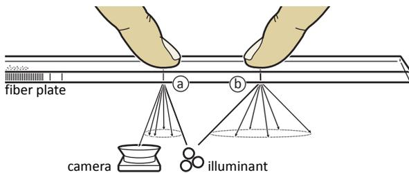
**Figure 11:** The light that comes back down the fiber is subject to same ring diffusion that we described earlier in terms of projection. While the camera will see reflections off the fiber plate’s surface at location (a), reflections from location (b) will be invisible, because the camera does not sit on the same ring.
