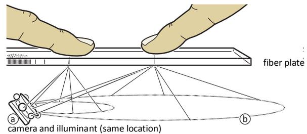
**Figure 13:** (a) Placing camera and illuminant in the same location causes the returning, ring-diffused light to always hit the camera. The farther away the finger, however, the less intense such reflections appear as they spread along increasingly large rings (b).
