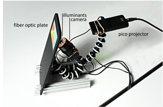
**Figure 12:** This earlier prototype placed the illuminant *around* the camera to approximate a shared location of camera and light source. Camera and illuminant were tilted with respect to the screen to prevent the camera from seeing the reflection of the illuminant in the fiber optic plate (hotspot).
