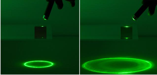
**Figure 7:** Pointing a laser at a fiber optic plate causes it to diffuse incident light into a ring. The angle of incident light thereby determines the radius of the ring, here small and large. The shown fiber optic bundle contains large-diameter fibers (1mm) and rests 5cm above a table surface.
