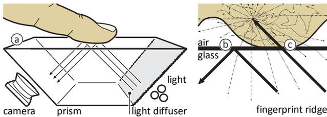
**Figure 5: (a) Optical fingerprint scanners produce crisp contrast between fingerprint ridges and valleys using a prism. (b) Rays from the illuminant are totally reflected at the prism surface, causing such locations to appear *bright* as the camera sees directly into the light source. (c) Light escapes the prism (i.e., the reflection is frustrated) where fingerprint ridges touch the surface, causing ridges to appear *dark*.**
