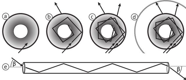
**Figure 8:** Each fiber diffuses parallel incident light into rings. (a) A fiber viewed top-down. (b) A ray enters the fiber and bounces down the fiber in a rotary pattern. (c) A parallel, but slightly offset ray exits into a different azimuth direction. (d) This variation in azimuth causes a ring, because (e) all rays have a constant exit angle with respect to the fiber.
