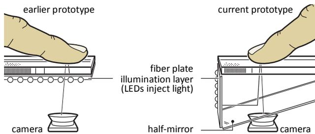
**Figure 14: Fiberio evenly illuminates the entire surface, creating one even reflection to see fingerprints across the whole surface. (left) An earlier prototype used Acrylight LED below the fiber plate. (right) Our current prototype uses a half-mirror that reflects illuminations from the side.**
