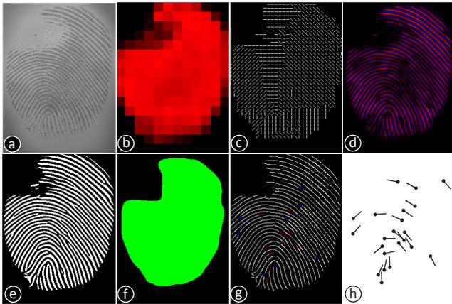
**Figure 16: Fingerprint processing pipeline (images are cropped). (a) Raw image, (b) areas of high standard deviation, (c) flow field, (d) Gabor filter, (e) binarized fingerprint, (f) mask, (g) skeleton and (h) extracted locations and orientations of all fingerprint features.**
