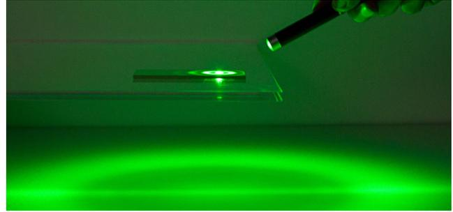
**Figure 9:** A fiber plate with a multitude of very small-diameter fibers ( $6\mu\text{m}$ ) blurs ring diffusion, which scatters the incoming light into all directions. This is the basis for good light diffusion, which we need to produce an image on a touchscreen. The fiber plate rests 5cm above the table. The image on the plate is visible even from extreme angles.
