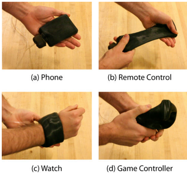
Figure 14: The ShapePhone mobile device can be formed into different jammed shapes.
